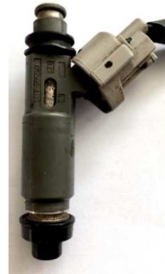
Figure 3. Fuel injector Denso 195500-3110.
